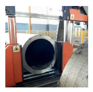
**Qualy**tube is provided by a band saw in order to prepare test coupons for further testing in external testing laboratories, qualified and approved by **Qualy**tube and certified in a accordance to ISO 17025.
